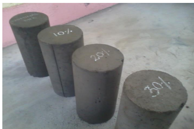
Figure 2 Replacing the cement with Bentonite in cylinder.
