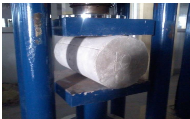
Figure 4 Tensile strength of bentonite powder in 28 days
