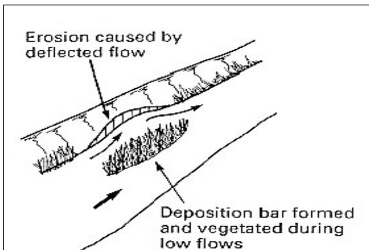
Figure 7 Erosion due to deflected flow by river island [21].
