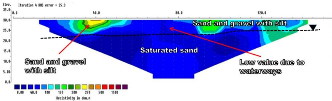
Figure 3 The electrical Resistivity Profile for Line 1 of Sungai Perak.
