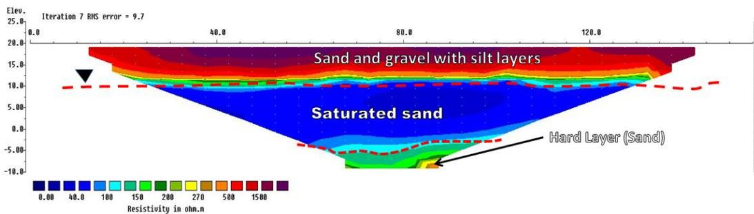
Figure 5 The electrical Resistivity Profile for Line 3 of Sungai Perak.
