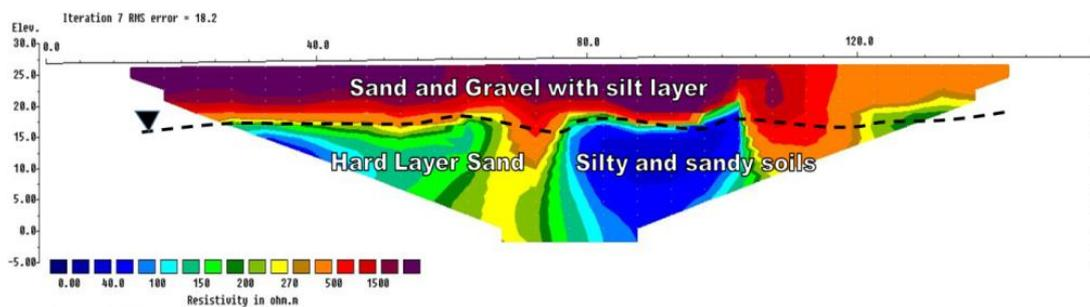
Figure 6 The electrical Resistivity Profile for Line 4 of Sungai Perak.
