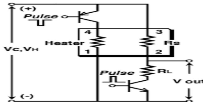
**Figure 2** Basic measuring circuit and pinout configuration for TGS 2442
