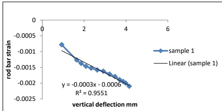
Figure 13: The timber vertical deflection vs. rod bar strain in post-tensioning process
