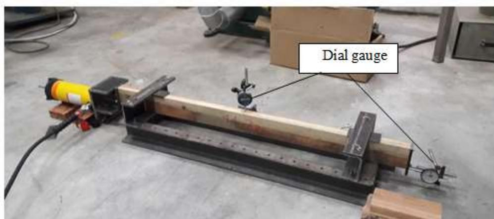
**Figure 5:** The dial gauge position in total system of post-tensioning
