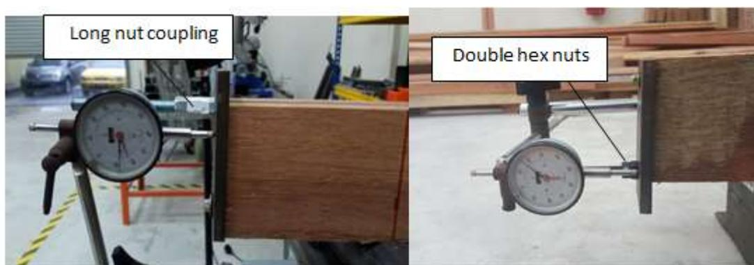
**Figure 11:** Long nuts coupling and double hex nut
