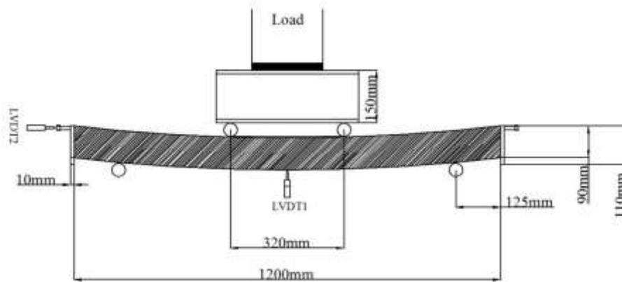
**Figure 6 b)** Second step is to release the nuts at rod bar then start applying load until the suitable deflection.
