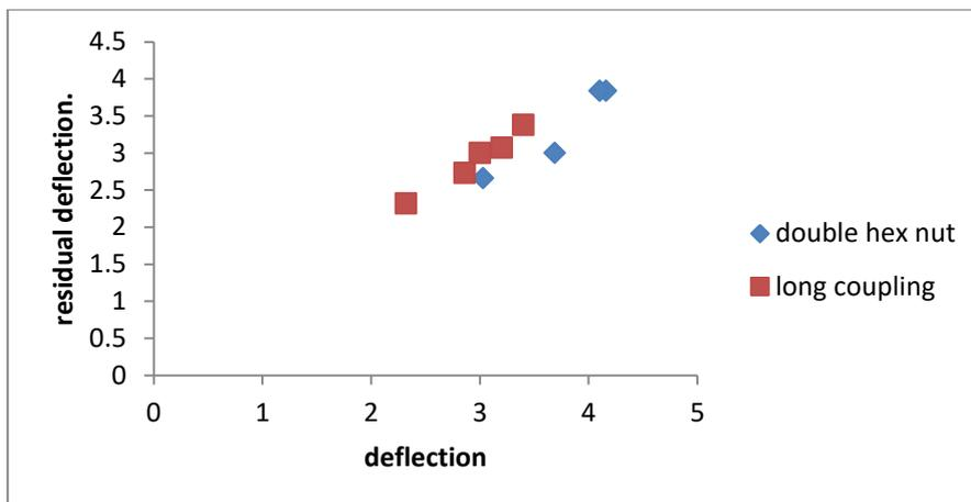
**Figure 10:** Correlation between deflection and residual deflection for two types of rod bar (silver color with long coupling nut and black color with double hex nut)
