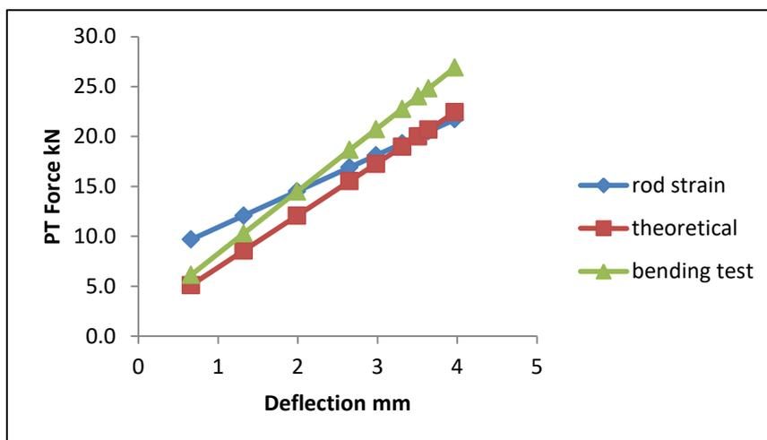
**Figure 15:** PT estimation in three methods (rod strain. bending test. theoretical)
