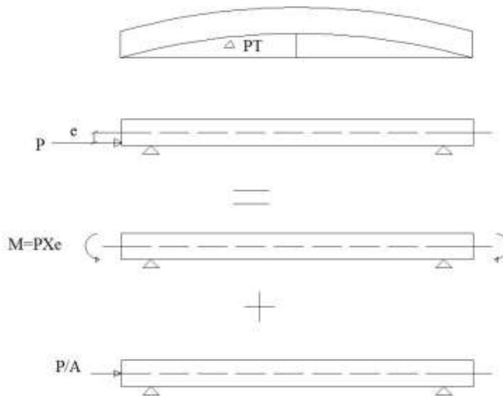
**Figure 1:** Post-tensioning force components
