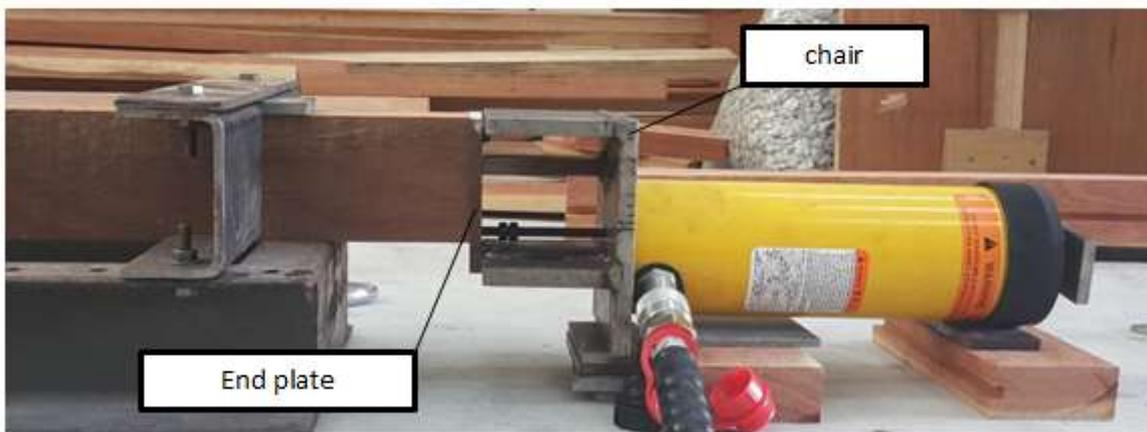
Figure 3: The chair part which used at the end of beam and end plate
