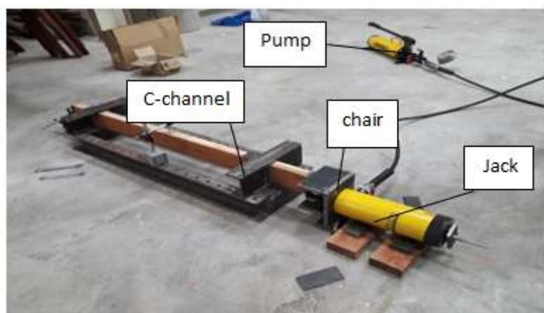
**Figure 4:** The total system of post-tensioning
