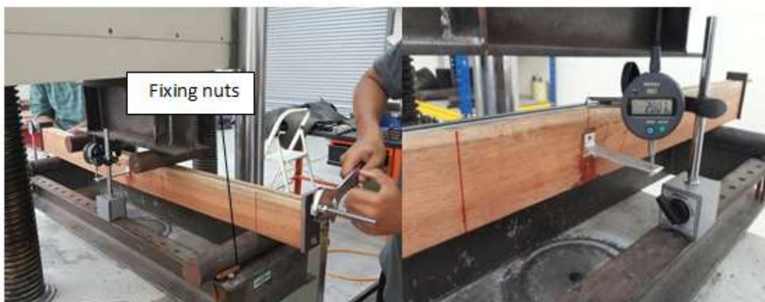
**Figure 8:** Fixing the post-tensioning force
