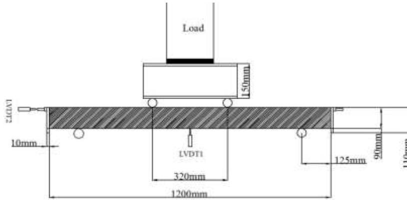
**Figure 6 a)** First step is putting the beam timber specimen upside down at universal testing machine
