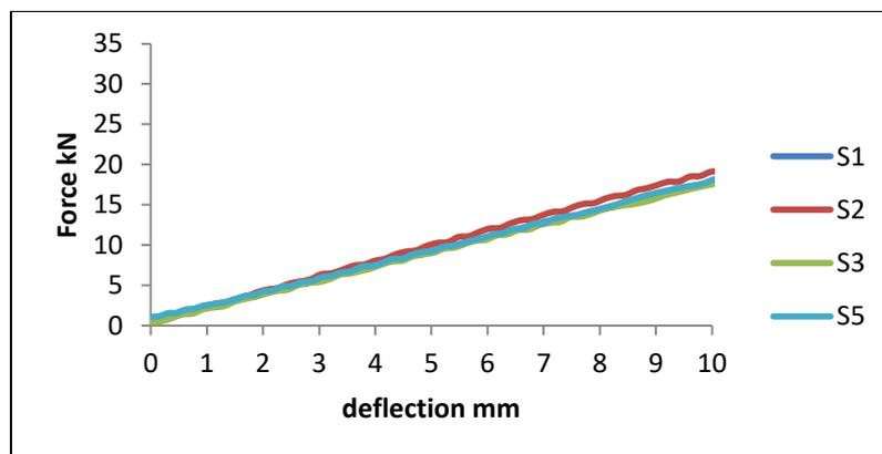
Figure 14: Experimental point load corresponding to deflection at range (10mm) for four samples.
