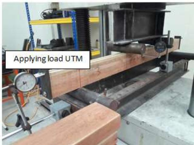
**Figure 7:** The process of post-tensioning by bending using universal testing machine
