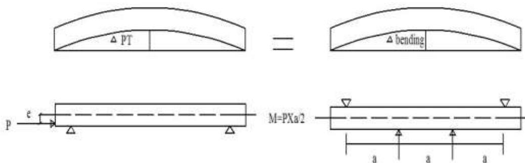
b) Similar deflection due post-tensioning force and 4 point bending.
