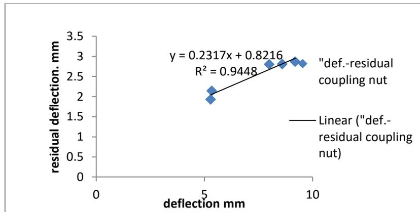
Figure 12 Correlation between deflection and residual deflection for silver rod bar using coupling nut.
