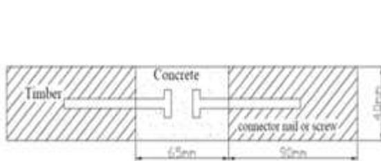
Figure 2 Push out test specimen plan view for single timber (T1)
