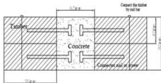
Figure 3 Push out test specimen plan view for double timber (T2)
