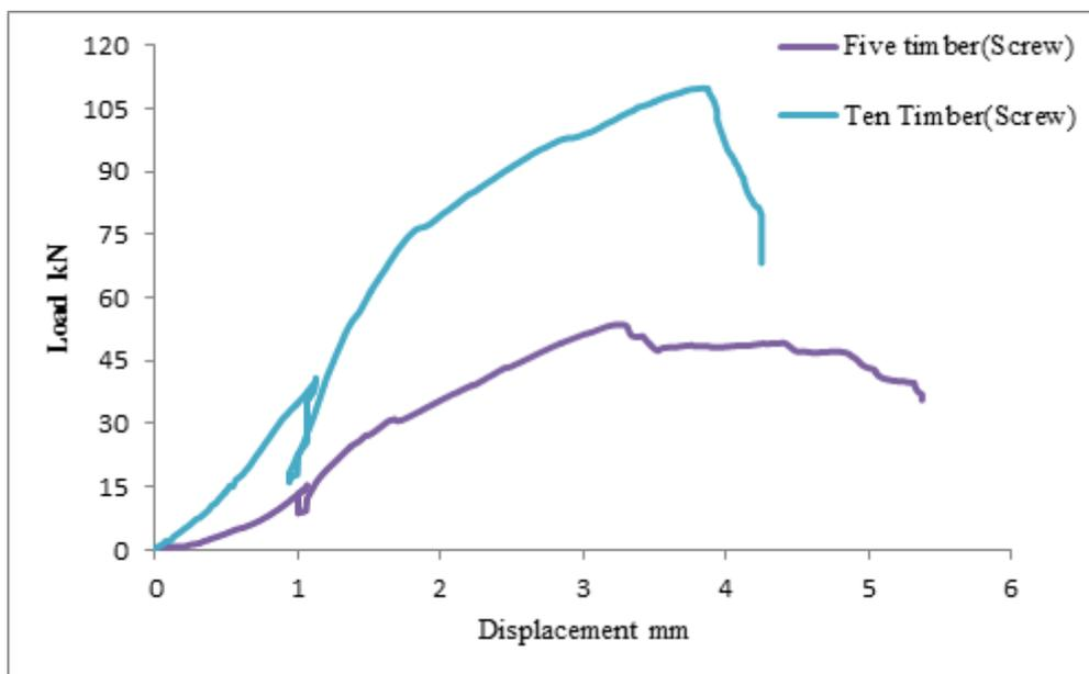
**Figure 12**: Test result of type (B) screw connectors for 5 and 10 timber
