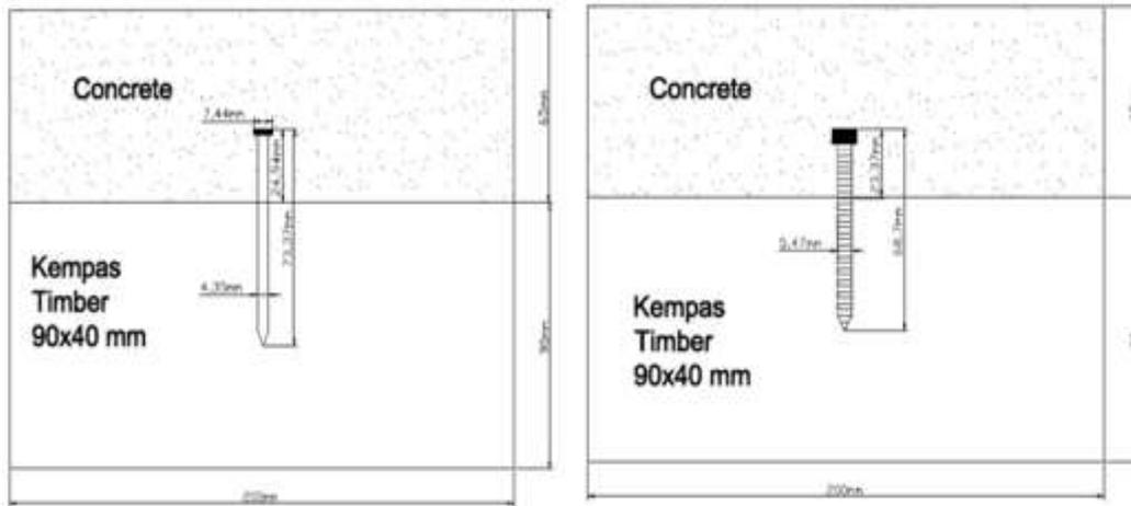
Figure 1: Details of nail and screw connectors
