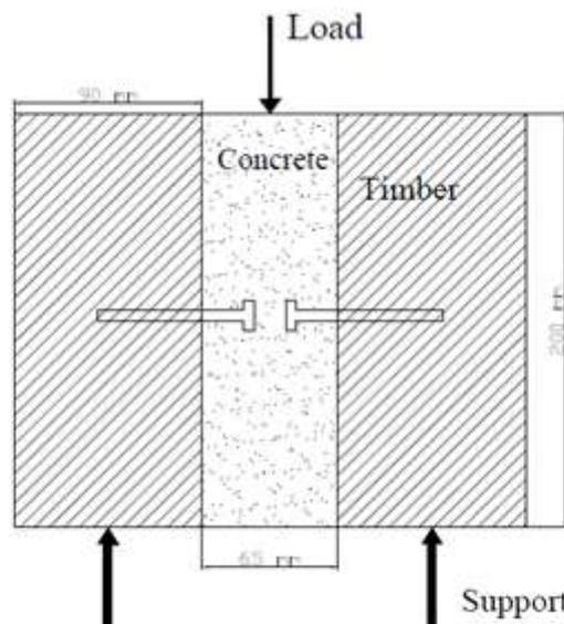
**Figure 11** Push out test specimen typical side elevation for single timber (T1)
