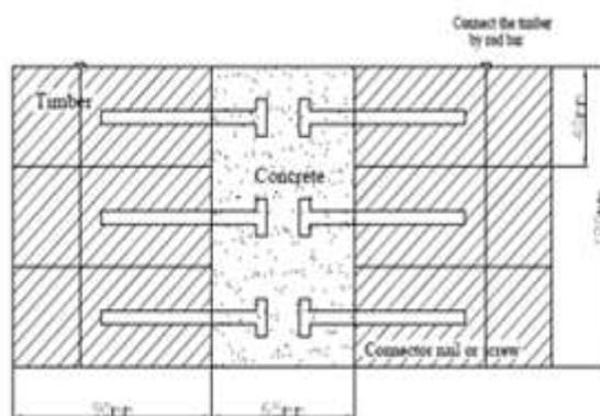
Figure 4 Push out test specimen plan view for Triple timbers (T3)
