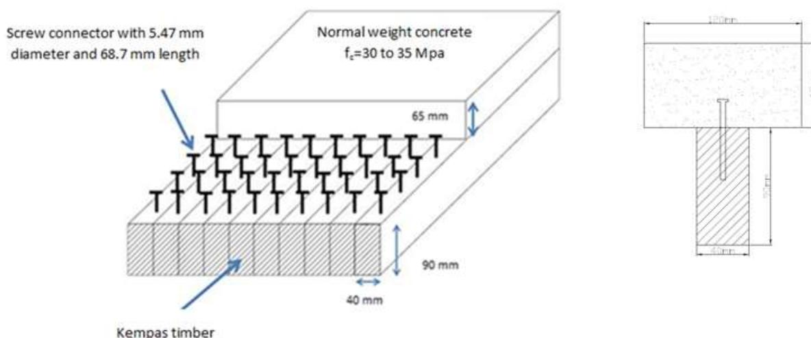
**Figure 16** Cross section for Timber concrete composite (TCC) deck(Left) and Single TCC1(T section) Right.
