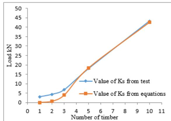
Figure 15: Slip modulus (Ks) versus number of screw connector.
