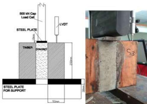
Figure 5 : Experiment set-up for push out test
