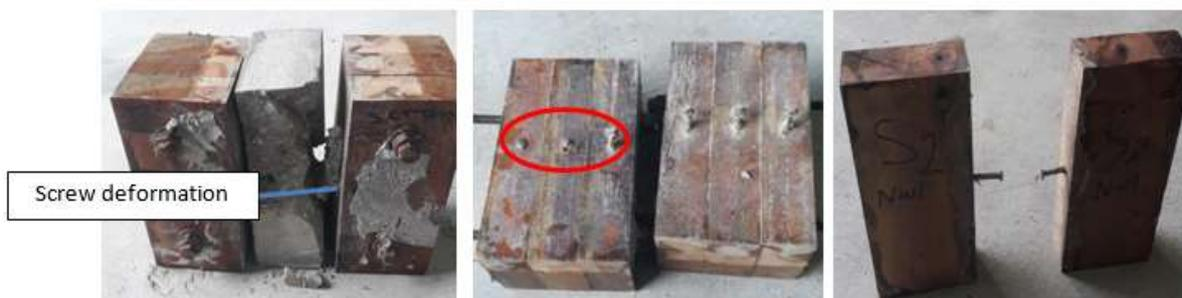
**Figure 7:** Type (B) Screw specimen after testing (shear deformation)
