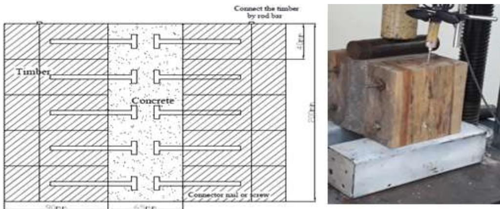
Figure 13 Push out test specimen plane view for 5 timbers (T5)
