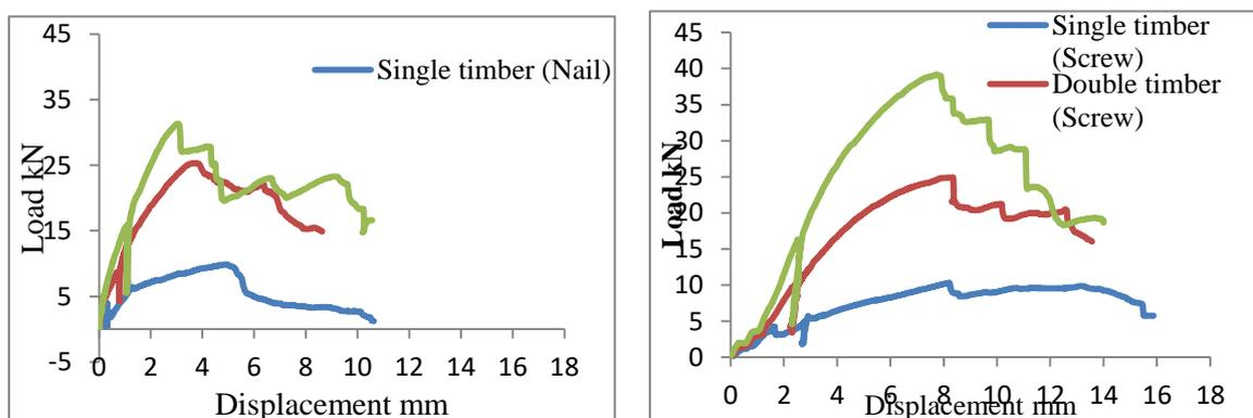
**Figure 10:** Test result of Type A nails (Left) and Type B screws (Right) connectors
