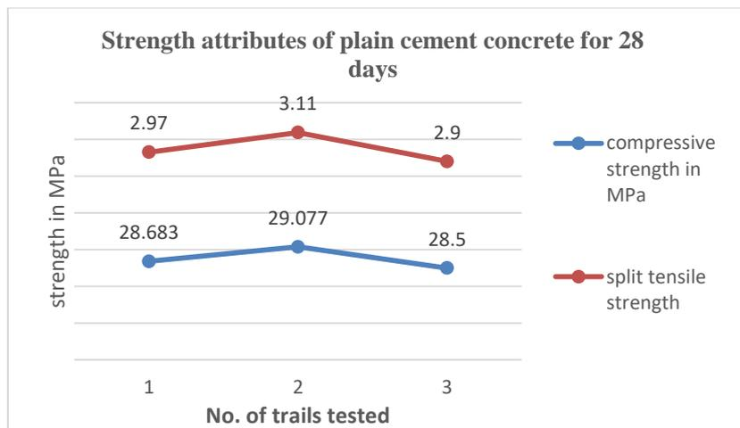
**Figure 4:** Strength attributes of plain cement concrete for 28 days
