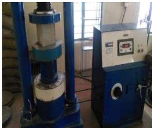
**Figure 2:** compression testing of specimen
