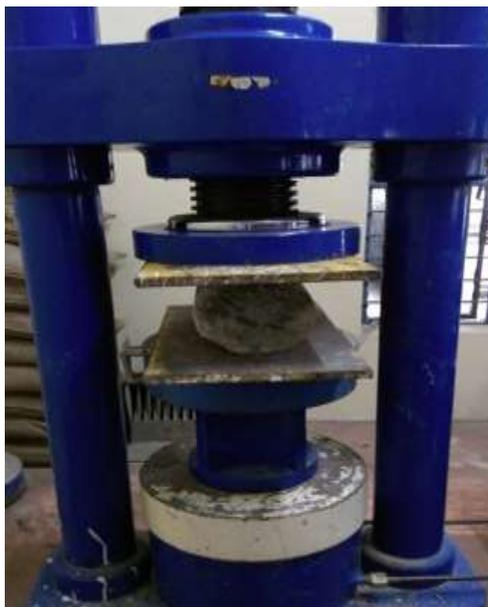
**Figure 3:** Split Tensile test on cylinder
