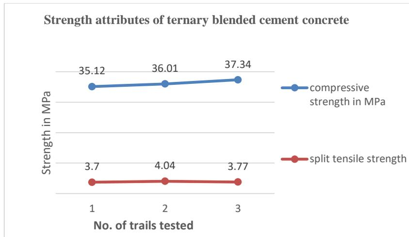
**Figure 5** Strength attributes of ternary blended cement concrete for 28 days
