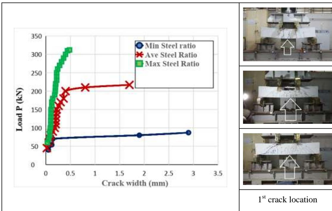
Figure 22 Load-first crack width for the specimens of Group B
