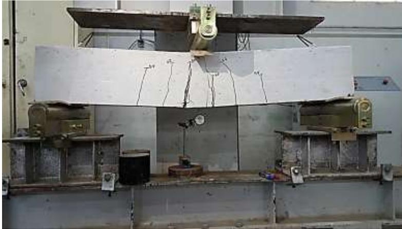
**Figure 10** Cracks propagation for the beam 1P-min
