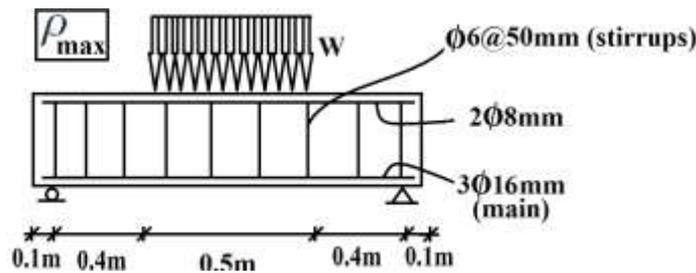
Figure 9 Reinforcement, geometry and loading of the beam Dist-max
