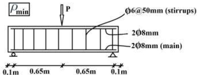
**Figure 1** Reinforcement, geometry and loading of the beam 1P-min
