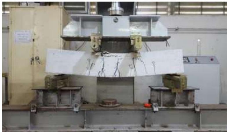
**Figure 13** Cracks propagation for the beam 2P-min
