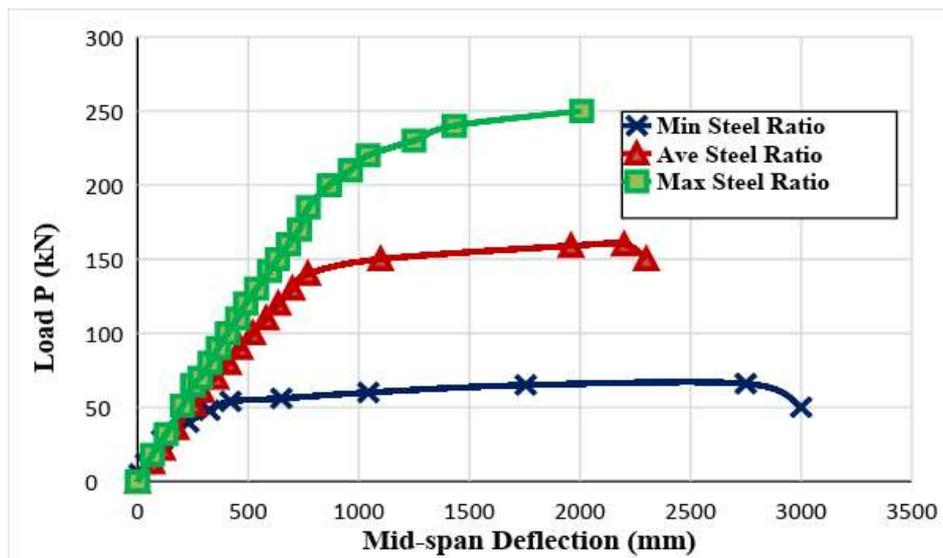
Figure 18 Load-midspan deflection for the specimens of Group A
