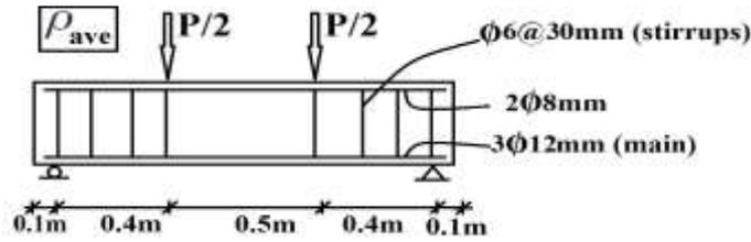
Figure 5 Reinforcement, geometry and loading of the beam 2P-ave
