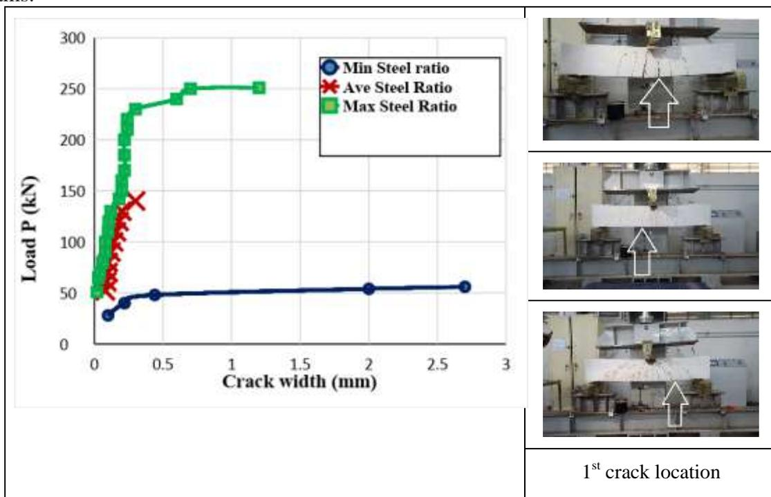
Figure 21 Load-first crack width for the specimens of Group A
