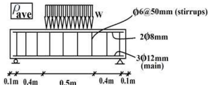
Figure 8 Reinforcement, geometry and loading of the beam Dist-ave
