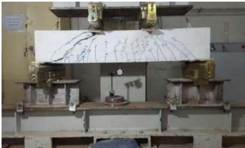
**Figure 15** Cracks propagation for the beam 2P-max
