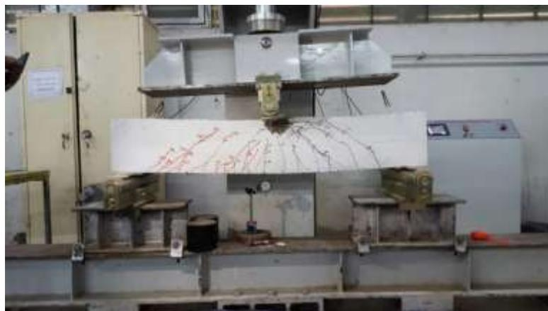
**Figure 12** Cracks propagation for the beam 1P-max
