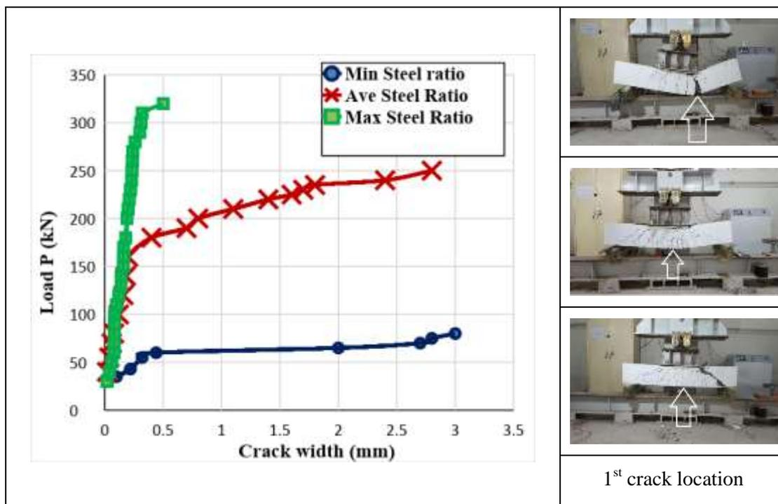
Figure 23 Load-first crack width for the specimens of Group C
