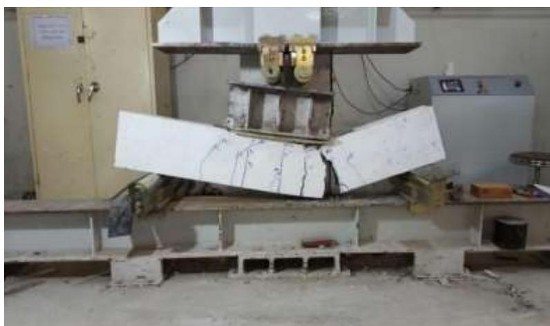
**Figure 16** Cracks propagation for the beam Dist-min
