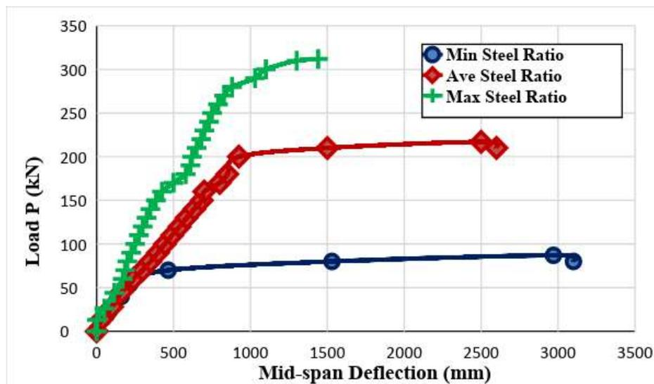
Figure 19 Load-midspan deflection for the Group B beams
