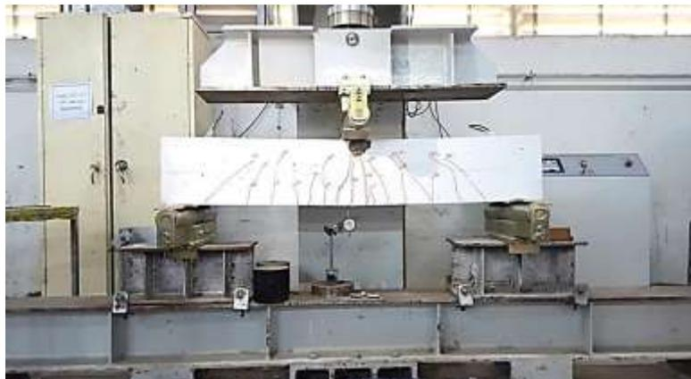
**Figure 11** Cracks propagation for the beam 1P-ave
