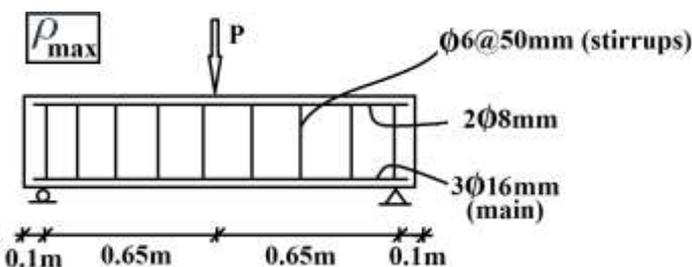
**Figure 3** Reinforcement, geometry and loading of the beam 1P-max
