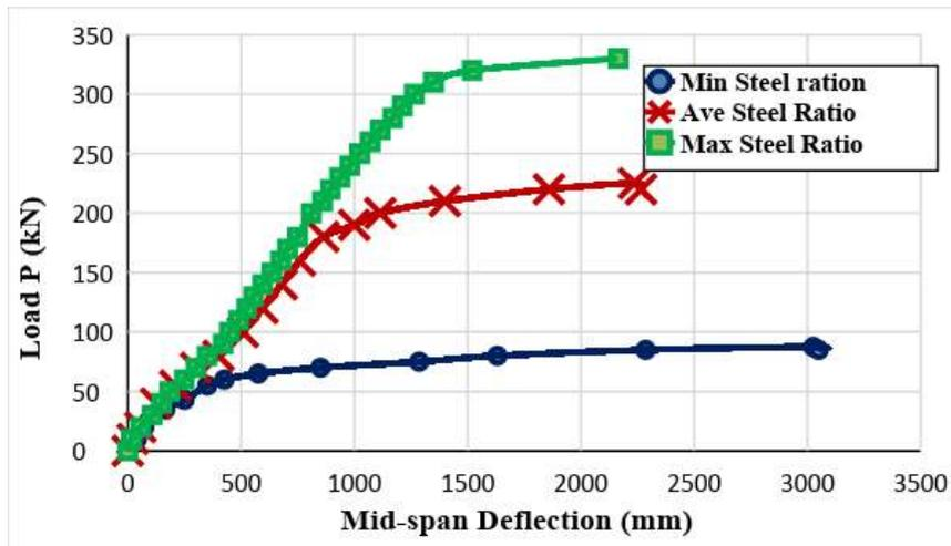
Figure 20 Load-midspan deflection for the specimens of Group C
