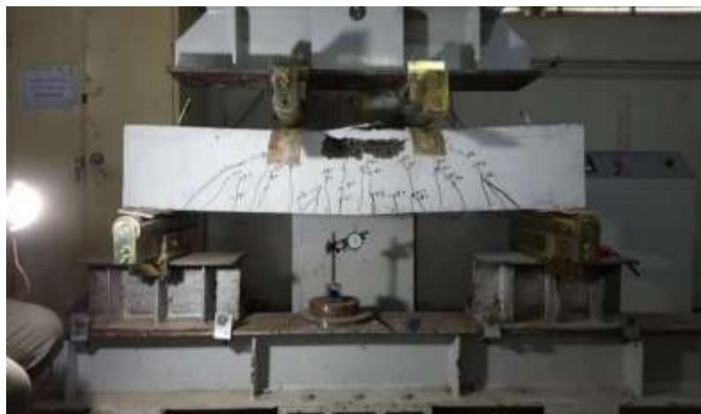
**Figure 14** Cracks propagation for the beam 2P-ave
