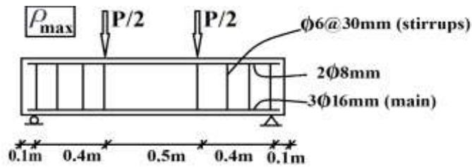
Figure 6 Reinforcement, geometry and loading of the beam 2P-max
