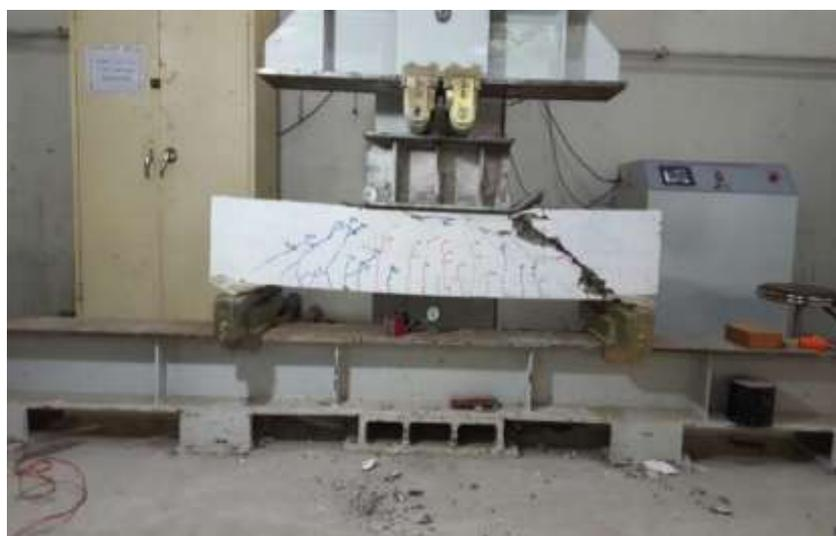
**Figure 18** Cracks propagation for the beam Dist-max
