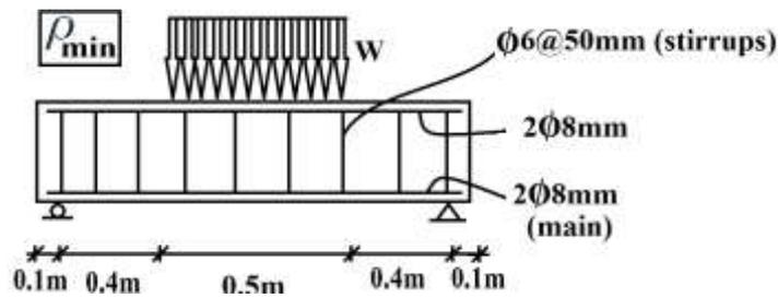
Figure 7 Reinforcement, geometry and loading of the beam Dist-min
