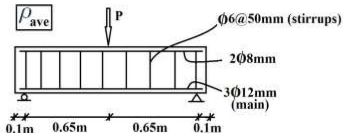
**Figure 2** Reinforcement, geometry and loading of the beam 1P-ave
