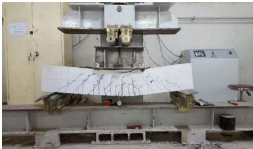
**Figure 17** Cracks propagation for the beam Dist-ave
