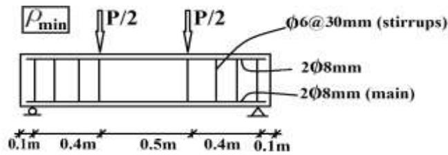
Figure 4 Reinforcement, geometry and loading of the beam 2P-min
