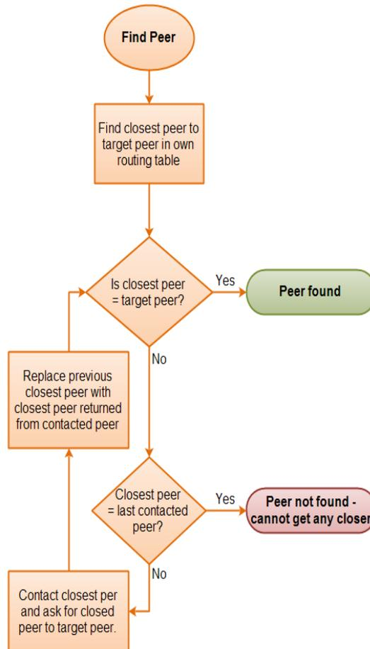
**Figure 3** The peer-to-peer routing workflow
