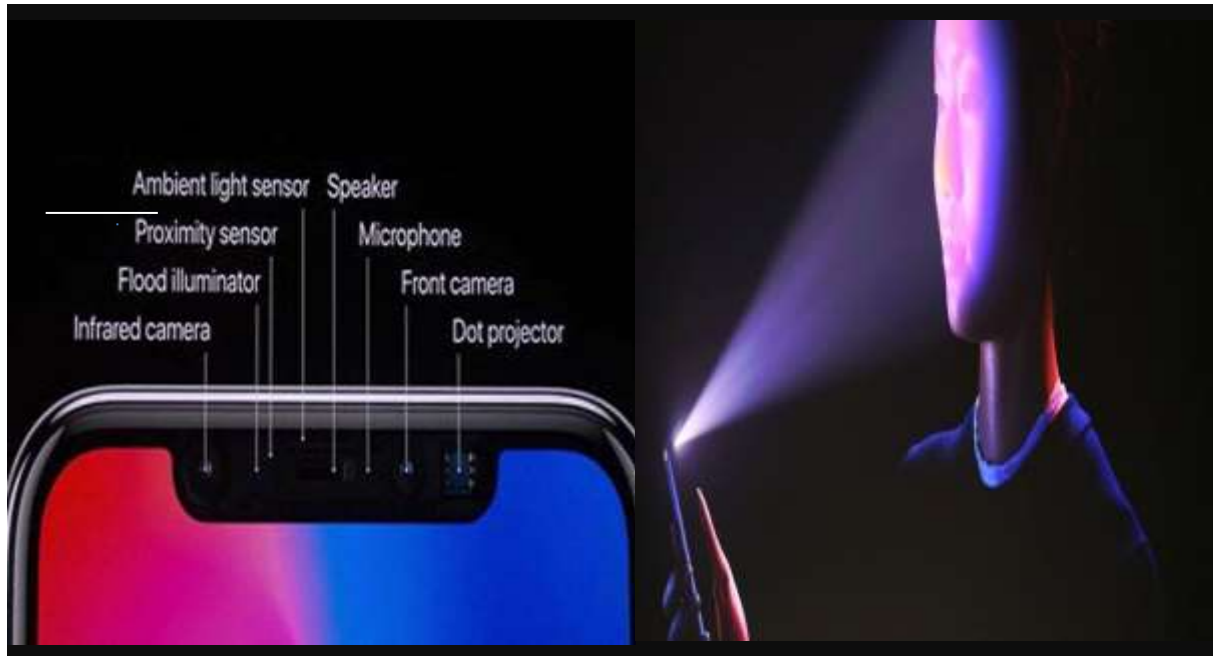
Figure 8 Depth Camera Area
