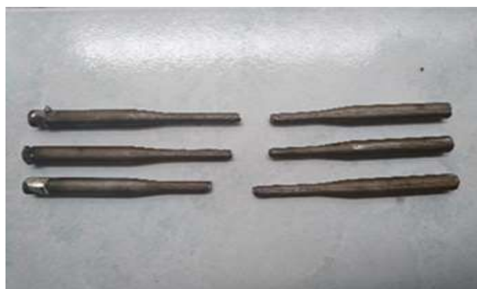
Figure 5 Speciment after tensile testing
