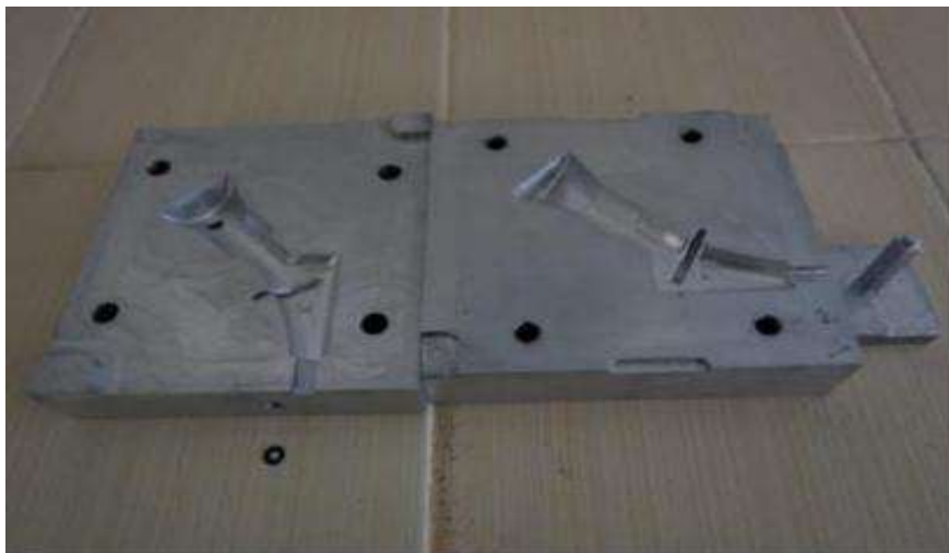
Figure 2 Metal dies of investment casting
