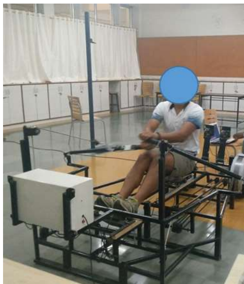
Figure 3 A subject performing the experiment of the re-designed rowing simulator
