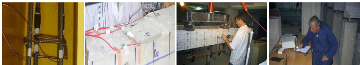
Figure 3 The installation of electronic strain gauges for measuring deformations in concrete and reinforcement, the measurement of deformations with mechanical strain gauge, data logger and Watson bridge for measuring deformations with electronic strain gauge
