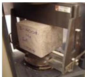
Figure 6 Testing of tensile splitting strength in the laboratory
