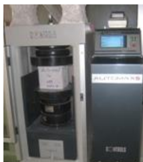
Figure 4 Testing the compressive strength of concrete in the laboratory
