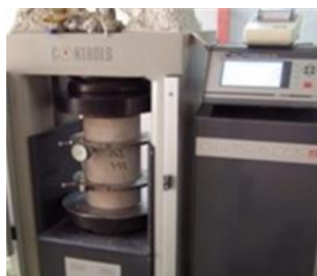
Figure 5 Determination of the modulus of elasticity in the laboratory
