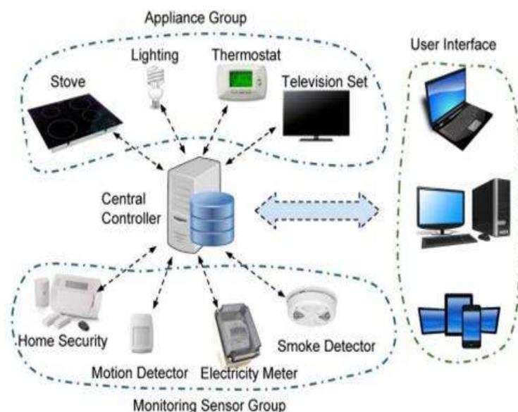
**Figure 1** IoT based smart home security
